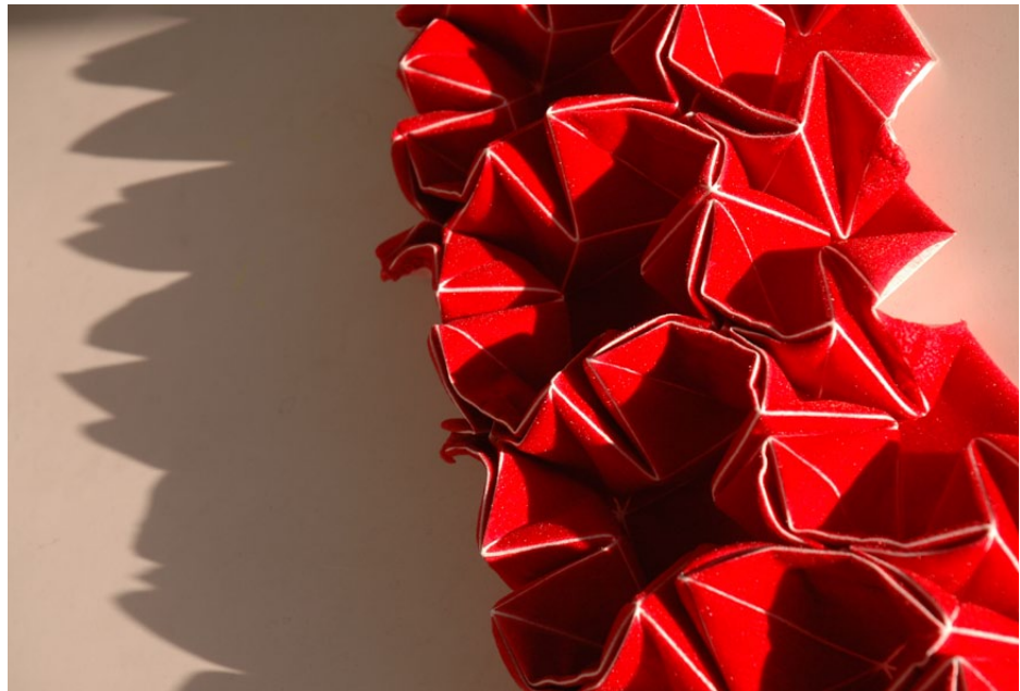
Figure 1: Deployable textile structure, silk-screen printed and hand folded polyesther.
